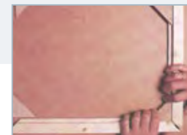
Accurately insert corner plates, finger tight, one per bar, then assemble frame.
